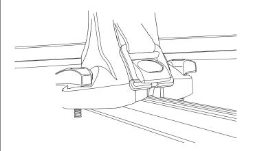
8. Pull the end of the attachment straps to secure the surfboard to the carrier. Make certain all mounting hardware is secure, then tighten as necessary. NOTE: Be careful not to overtighten the attachment straps as you could damage the surfboard.
