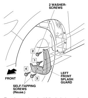
5. Turn the steering wheel fully clockwise, and repeat steps 2 through 4 to install the right front splash guard.
