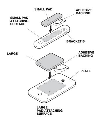
Using isopropyl alcohol on a shop towel, clean the four plates where the large pads will attach. Remove the adhesive backings from the large pads, and attach them to the plates. 6. Under the roof box, insert a bolt through bracket B, through the plate, and into the predrilled hole in the bottom of the roof box. Install bracket B and the plate with the pads facing each other.
