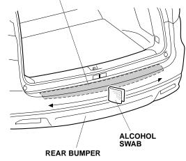
5. Using a spray bottle with the 3M protective tape application solution, spray the area where the rear bumper applique will attach. Spray some solution on your hands.
