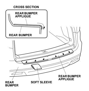
15. Using a shop towel, wipe up the 3M protective tape application solution. Allow the rear bumper applique to dry thoroughly.
