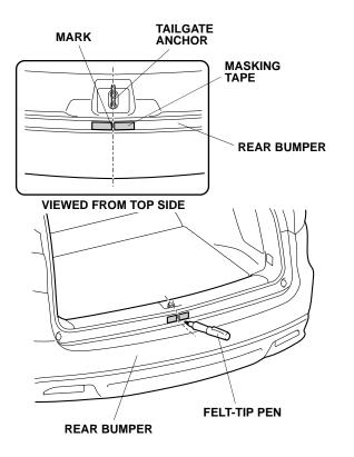
2. Align the rear bumper applique to the rear bumper and check the rear bumper applique installation position.
