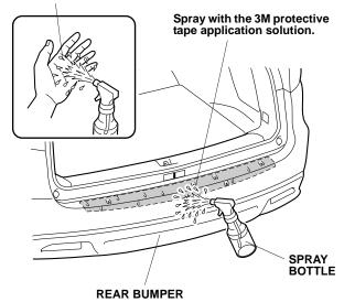
6. Remove the adhesive backing from the side of the rear bumper applique with the 3M mark.
