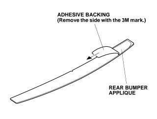
7. Spray the rear bumper applique with the 3M protective tape application solution.
