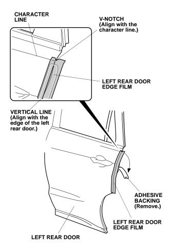
19. Align the vertical line on the left rear door edge film to the edge of the left rear door. While applying light pressure, carefully remove the adhesive backing. 20. Starting from the center and working outward, use the soft sleeve to smooth out the left rear door edge film. Move the soft sleeve in one direction only.
