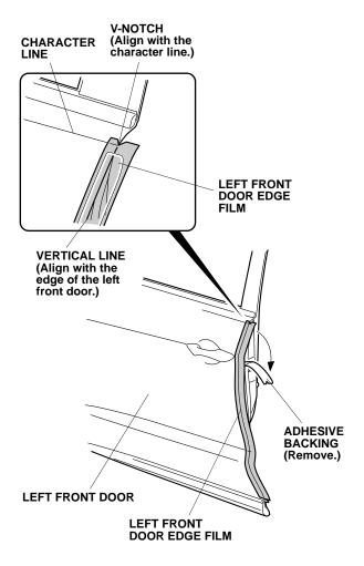
Align the vertical line on the left front door edge film to the edge of the left front door. While applying light pressure, carefully remove the adhesive backing. 11. Insert the applicator into the soft sleeve.
