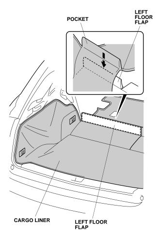
6. Secure the cargo liner to the left rear seat back with the fasteners. If the vehicle is equipped with a rear seat cover, release one fastener, fasten the cargo liner to the seat-back, then secure the seat cover to the cargo liner.
