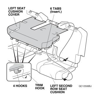
9. Set the left seat cushion cover under the seat belt buckle as shown. Insert the left seat cushion cover between the left second row seat-back and left second row seat cushion, and secure the fasteners to the left second row seat cushion.
