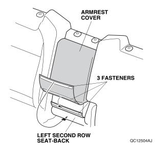
6. Secure the fastener to the bottom of the left second row seat-back.
