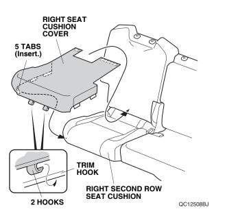
11. Insert the right seat cushion cover between the right second row seat-back and right second row seat cushion, and secure the fasteners to the right second row seat cushion.
