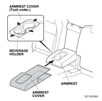
5. Raise the armrest. Pull the armrest cover between the armrest and left second row seat-back, and secure the fasteners on the armrest cover as shown.
