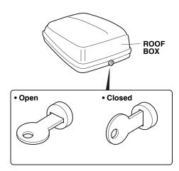
**Locking:** Press down on the lid. There should be an audible click. Be sure the lid is latched by attempting to lift the lid. Turn the key clockwise to lock the roof box. Remove the key while not in use. Be sure the straps are not outside the roof box.
