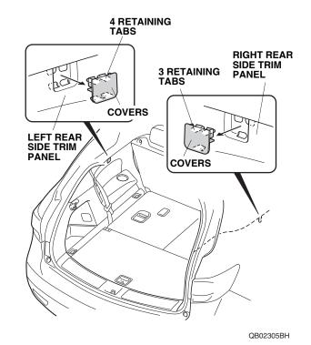
9. Install the cargo cover into the recess in the right rear side trim panel, then compress the cargo cover, and install it in the left rear side trim panel.
