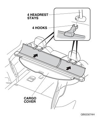
11. Attach each hook of the cargo cover to the left and right catches.
