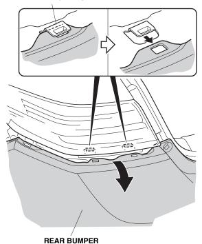
With the help of an assistant, remove the rear bumper (four retaining tabs). Place the rear bumper on a blanket to prevent damage.
