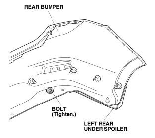
14. Repeat steps 5 through 13 to install the right rear under spoiler on the right side of the rear bumper.
