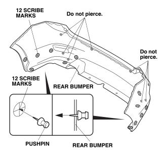
3. While wearing eye protection, drill the 12 pierced marks with a 3 mm drill bit. Enlarge the holes with a 10 mm drill bit.
