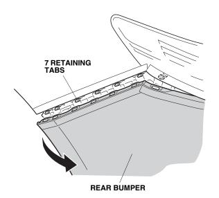
Release two retaining tabs on each side.
