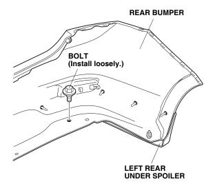
9. Loosely install a clip holder onto each clip on the left rear under spoiler. Do not tighten the clips at this time.
