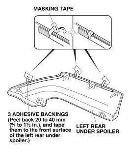
7. Insert the four clips on the left rear under spoiler into the four holes in the bumper. Secure the left rear under spoiler with a bumper clip and washer from the kit.
