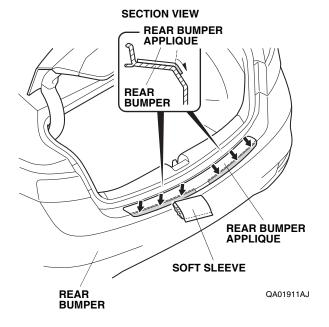
13. Using a shop towel, wipe away the excess 3M protective tape application solution. Allow the rear bumper applique to dry thoroughly.
