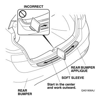
Slowly remove the protective film from the top of the rear bumper applique. Remove the protective film by pulling it slowly and horizontally; do not pull it vertically.
