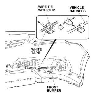
22. Secure the vehicle harness to the front bumper.
