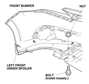
13. Loosely install one clip holder onto each clip on the left front under spoiler. Do not tighten the clips at this time.
