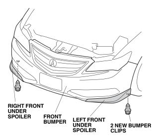
24. Using a rubber roller, apply firm pressure, especially at the ends, to set the adhesive.
