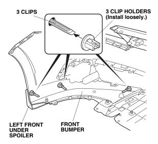
14. Slowly and carefully remove the adhesive backing from the left front under spoiler. Press and hold the front under spoiler against the front bumper with the palm of your hand for 30 seconds.
