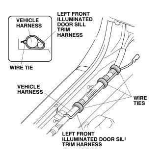
55. Plug the door sill trim harness 2-pin connector into the left front illuminated door sill trim harness 2-pin connector.
