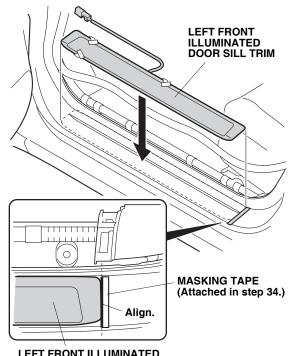
LEFT FRONT ILLUMINATED DOOR SILL TRIM 46. Attach the left front illuminated door sill trim to the vehicle panel by removing the three adhesive backings and pressing on the trim firmly with your hands.
