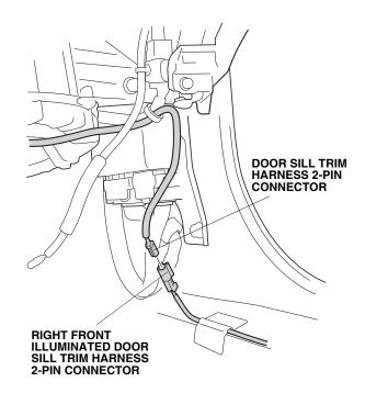
81. Secure the door sill trim harness 2-pin connector to the vehicle harness with one wire tie.
