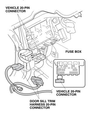
20. Attach the door sill trim harness 20-pin connector to the vehicle 20-pin connector.
