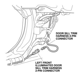
56. Bundle the excess door sill trim harness, and secure it to the vehicle harness with one wire tie.
