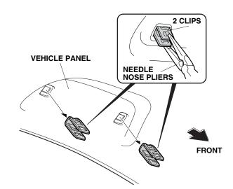
33. Reinstall the left grab rail with two clips. Reinstall the caps.
