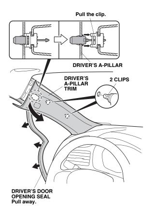
• To prevent clips from falling into the body panel area, carefully insert a shop towel between the driver's A-pillar and the driver's A-pillar trim.
