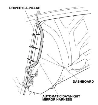
21. Align the green tape on the automatic day/night mirror harness with the vehicle clip, and secure the automatic day/night mirror harness to the vehicle harness with one wire tie as shown.
