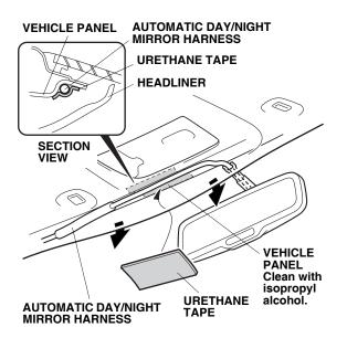
29. Secure the automatic day/night mirror harness to the vehicle panel with one urethane tape as shown. Be careful not to crease the headliner.
