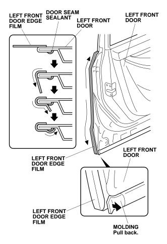
18. Using a shop towel, wipe the excess protective tape application solution from the left front door edge film. Allow the left front door edge film to dry thoroughly.
