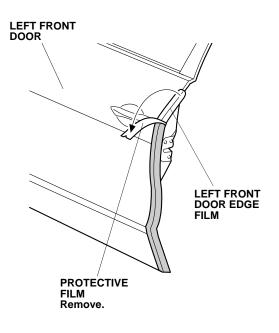
17. Starting from the center and working outward, use the soft sleeve to fold the left front door edge film inside the left front door as shown. Move the soft sleeve in one direction only. Do not damage the door seam sealant. Pull back the molding on the left front door.
