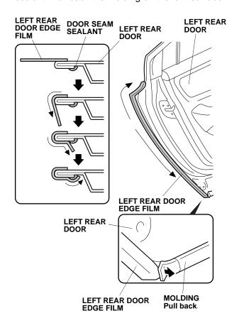
29. Using a shop towel, wipe the excess protective tape application solution from the left rear door edge film. Allow the left rear door edge film to dry thoroughly.
