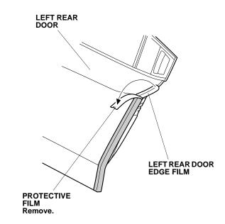
28. Starting from the center and working outward, use the sleeve to fold the left rear door edge film inside the left rear door as shown. Move the sleeve in one direction only. Do not damage the door seam sealant. Pull back the molding on the left rear door.
