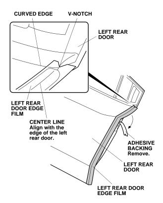
25. Align the center line on the left rear door edge film to the edge of the left rear door. While applying light pressure, carefully remove the adhesive backing.
