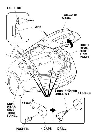
3. While wearing eye protection, drill two holes in the left and two holes in the right rear side trim panels. First drill with a 3 mm drill bit, then enlarge the holes with a 10 mm drill bit. To prevent damage to the inner panels, wrap tape around the end of each drill bit 10 mm away from the tip.
