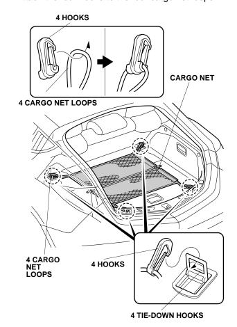
7. Secure the four cargo net hooks to the four tie-down hooks.
