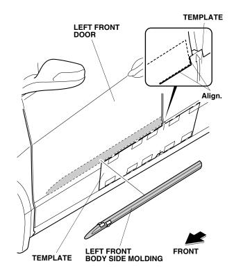
Peel back approximately 1½ to 2 inches of adhesive backing from each adhesive strip, and tape the ends to the front surface of the body side molding. Remove the small end pieces of adhesive backing.
