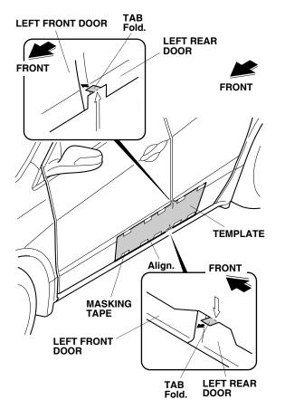
3. Align the template to the left front door and left rear door and attach it with pieces of masking tape as shown.
