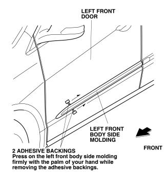
10. Using a rubber roller, apply pressure against the left front body side molding and roll from one end to the other.
