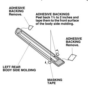
7. Align the left rear body side molding with the template and attach it to the left rear door as shown.
