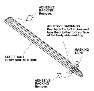
5. Align the left front body side molding with the template and attach it to the left front door as shown.
