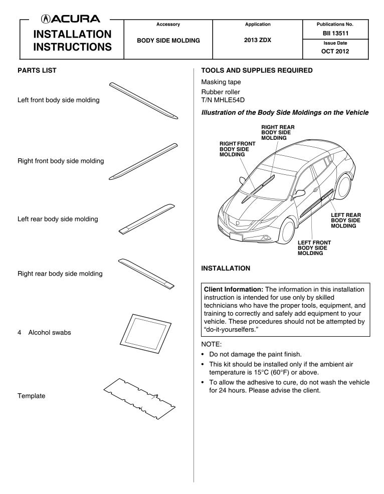
1. Using an alcohol swab, clean the areas where the left body side moldings will attach.
