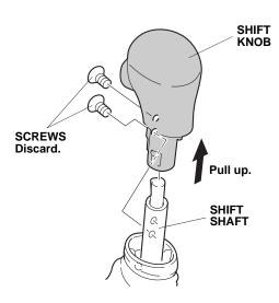
Install the select knob using the two new screws. Using a Torque screwdriver, torque the screws to 1.57 N·m (14 lb-in) Do not overtighten the screws.
