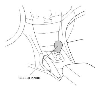
2. Lower the shift boot by pushing the two tabs in the positions shown.
