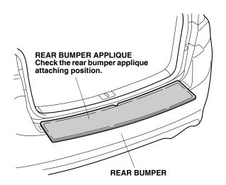
2. Remove the rear bumper applique. Using isopropyl alcohol on a lint-free shop towel, clean the rear bumper where the rear bumper applique will attach.
