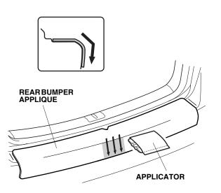
11. Use the applicator to apply the rear bumper applique to the rounded rear edge on the left side as shown. Start in the middle and work outward. Repeat for the right side.
