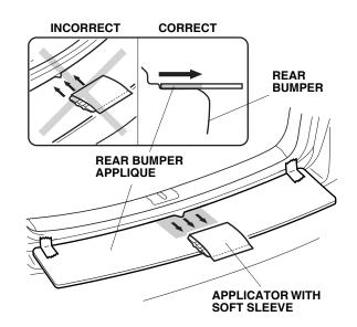
8. Starting from the center and working outward, use the applicator to smooth the rear bumper applique. Repeat on the right side. Stroke outward only.
