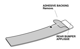
5. Generously apply the protective tape application solution to the adhesive side of the rear bumper applique.
