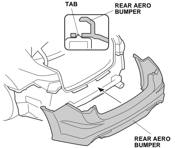
9. Secure the rear aero bumper to the vehicle by reusing the two bolts, ten self-tapping screws, two clips, and the two caps.
