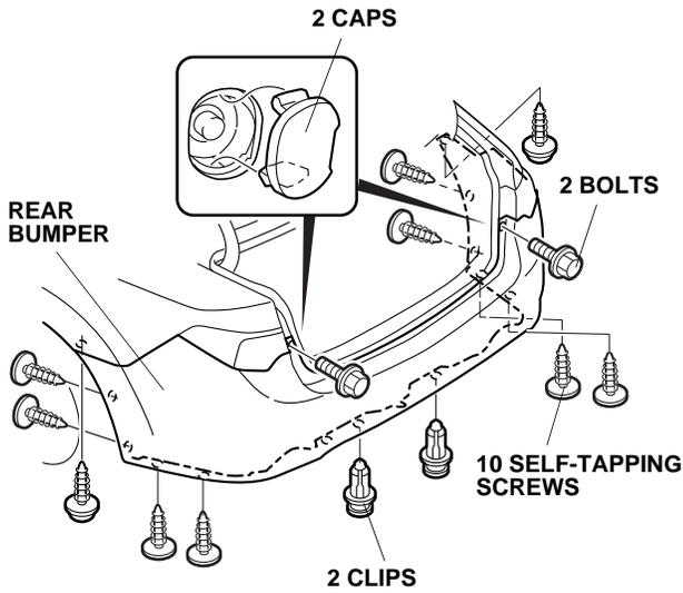
2. Remove the two clips and the ten self-tapping screws from the rear bumper.
