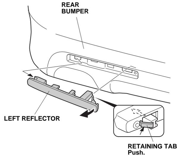
5. Transfer the left and right reflectors to the new aero bumper.
