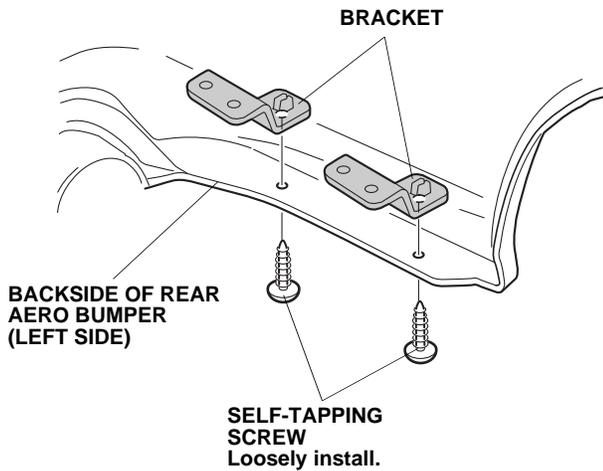
8. Fit the rear aero bumper in place on the vehicle.
