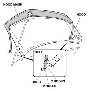
2. Secure the two hooks on the hood mask to the two holes in the hood.
