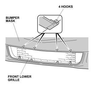
15. Secure four hooks on the bumper mask to the front lower grille.
