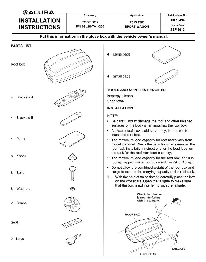
2. Open the roof box, and align the holes in the plate with thte mouting location at the forward crossbar. The plate is located at the front of the base of the roof box.
