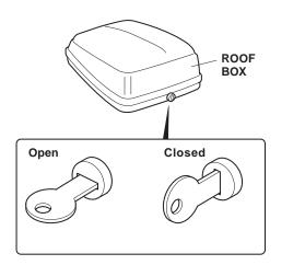
**Locking:** Press down on the lid. There should be an audible click. Be sure the lid is latched by attempting to lift the lid. Turn the key clockwise to lock the roof box. Remove the key while not in use. Be sure the straps do not dangle from the box.
