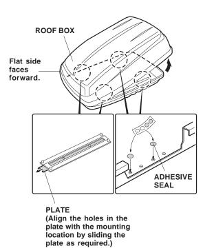
3. Attach an adhesive seal over each of the four unused mounting holes (two on each side) at the rear of the base of the box. The seals will help prevent water from entering the roof box. Then, remove the roof box from the crossbars.
