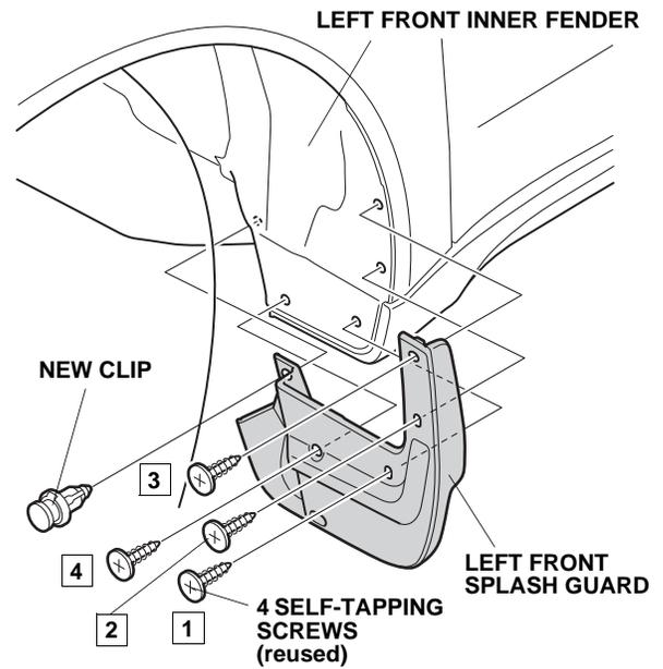
4. While holding the left front splash guard against the left front inner fender, tighten the four self-tapping screws in the order shown. Install the new clip. Make sure there is no gap between the left front splash guard and the vehicle. If there is, loosen the four self-tapping screws and the clip, adjust the splash guard to remove the gap, and retighten the fasteners.
