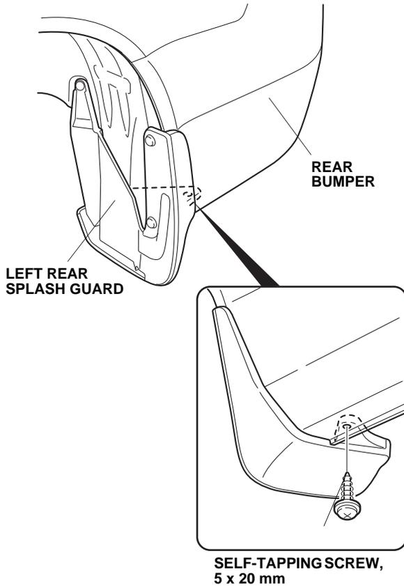
11. While holding the left rear splash guard against the rear bumper, tighten the four self-tapping screws in the order shown. Make sure there is no gap between the left rear splash guard and the vehicle. If there is, loosen the four self-tapping screws, adjust the splash guard to remove the gap, and retighten the screws.
