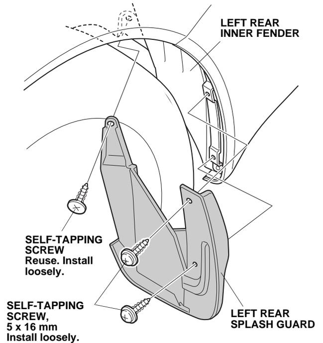
10. Secure the left rear splash guard to the rear bumper with a loosely-installed 5 x 20 mm self-tapping screw.
