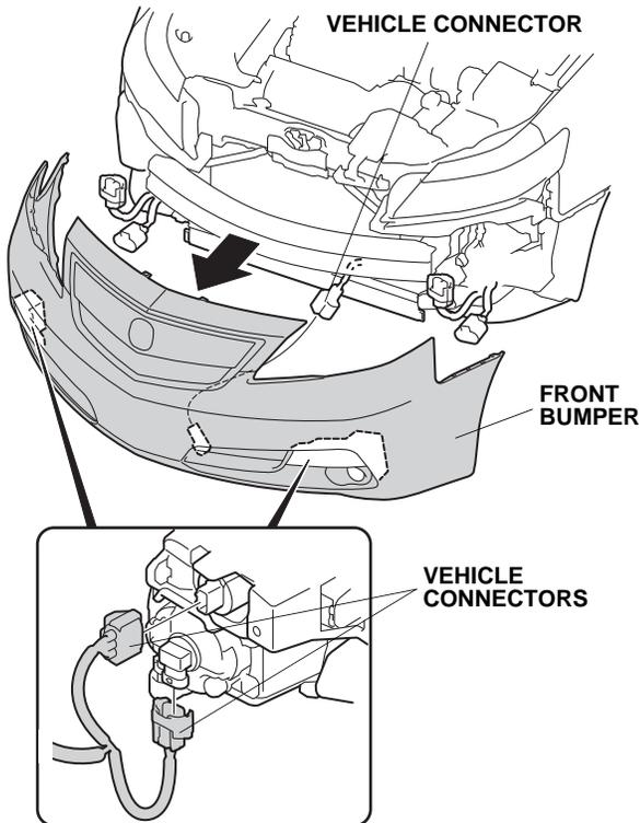
11. Unplug the vehicle connector, and remove the vehicle connector from the vehicle bracket.
