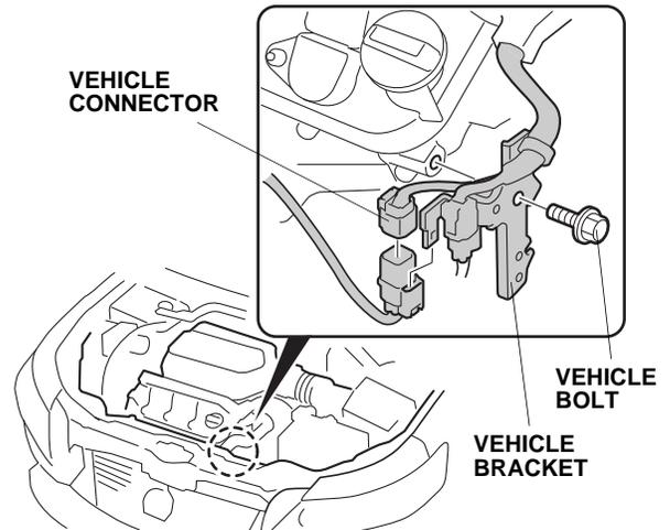
12. Remove the vehicle bolt, and release the vehicle bracket.
