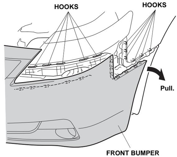
10. With the help of an assistant, remove the front bumper (unplug the five vehicle connectors). Place the front bumper on a blanket so it does not get damaged.
