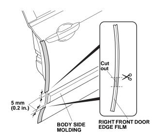
6. Continue to remove the adhesive backing while you align the centerline on the door edge film with the edge of the door.
