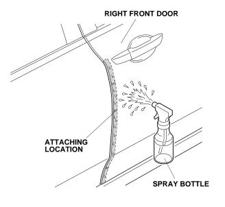
Open the right front door again. Measure 140 mm (5.5 in.) down from the bottom of the door glass outer weatherstrip, and mark the door.
