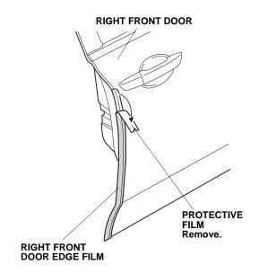
Starting in the middle of the door edge film and working outward, fold the door edge film around the door edge using your fingers. Move your finger in one direction. Attach the film over the seam sealant. Do not trim or damage the seam sealant.
