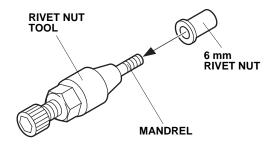
5. Insert the 6 mm rivet nut into the hole in the vehicle panel, and attach the hex wrench to the rivet nut tool.
