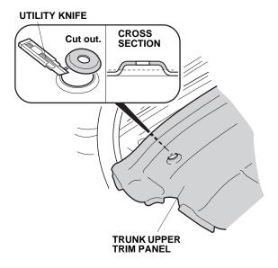
9. Make sure that the cargo hook bracket can be inserted into the hole in the trunk upper trim panel. If necessary, enlarge the hole in the trunk upper trim panel.
