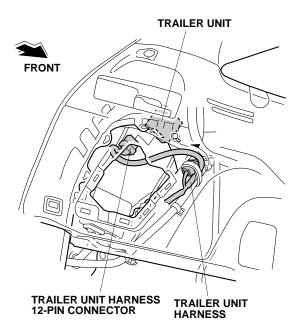
Secure the trailer unit harness to the vehicle harness with two wire ties.
