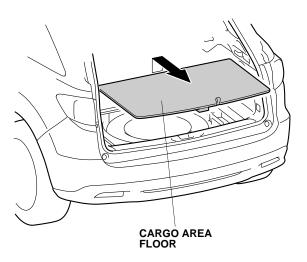
3. Remove the cargo area front floor lid (four clips).
