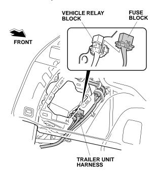
24. Secure the trailer unit harness to the vehicle harness with three wire ties.
