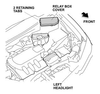
37. Plug the 20A fuse into the relay box as shown.
