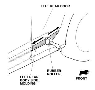
Turn the template over and repeat steps 1 through 12 to install the body side moldings on the right side of the vehicle.
