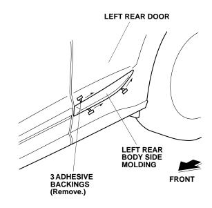
12. Using a rubber roller, apply pressure against the left rear body side molding and roll from one end to the other.
