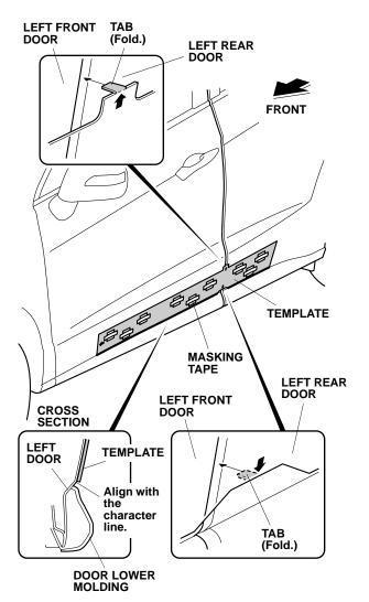
2. Align the template with the character line above the door lower molding, and attach the template to the left doors with strips of masking tape as shown.
