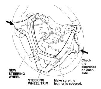
20. Install the two self-tapping screws into the new steering wheel.
