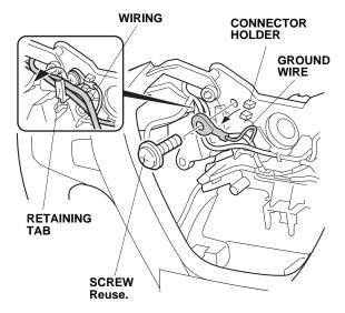
14. Remove the steering wheel trim by releasing the wiring from the seven retaining tabs.
