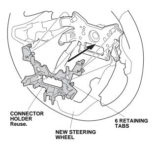
17. Position the steering wheel trim to the new steering wheel, and attach the wiring to the seven retaining tabs.
