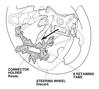
Install the connector holder on the new steering wheel.
