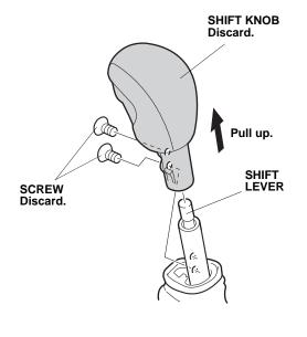
4. Install the new shift knob using the two new screws. Using a torque screwdriver, torque the screws to 3 N·m (18 lb-in). Do not overtighten the screws.
