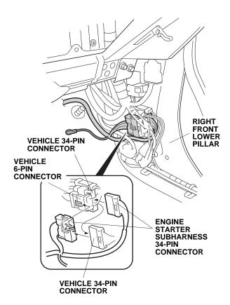
64. Unplug the vehicle 34-pin connector, and plug the engine starter subharness 34-pin connectors in between.
