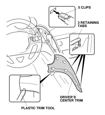
17. Remove the driver's lower dashboard cover (one self-tapping screw and nine clips). If equipped, unplug the A/C sensor (two retaining tabs).
