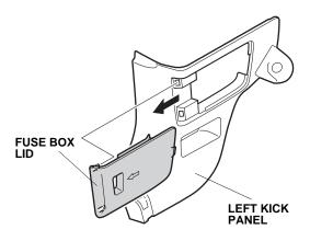
80. Install the 3A fuse included in the kit into the No. 33 slot in the fuse box.
