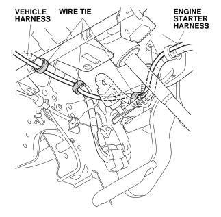
57. Secure the engine starter harness 6-pin connector (green) to the vehicle harness with one wire tie. Near the relays, secure the engine starter harness (white tape) to the vehicle harness with one wire tie.
