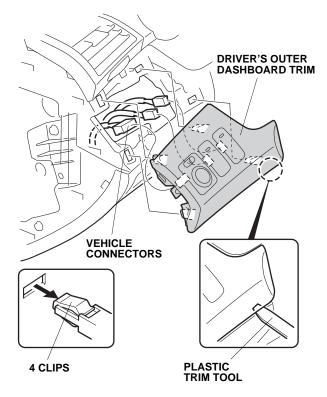
16. Using a plastic trim tool and a shop towel, remove the driver's center trim (five clips and three retaining tabs).
