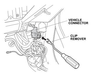
66. Remove the vehicle ground bolt. Attach the engine starter subharness ground terminal, and reinstall the vehicle ground bolt.
