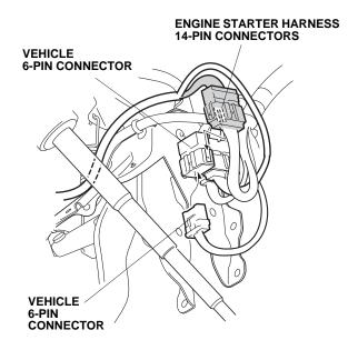
53. Reconnect the vehicle 6-pin connector.
