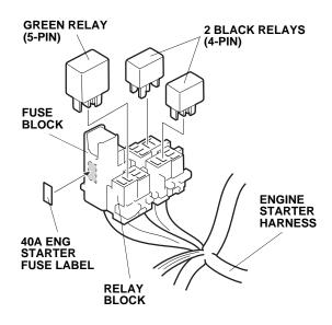
39. Using isopropyl alcohol on a shop towel, clean the fuse block where the fuse label will attach. Attach the 40A ENG STARTER fuse label to the engine starter harness fuse block.
