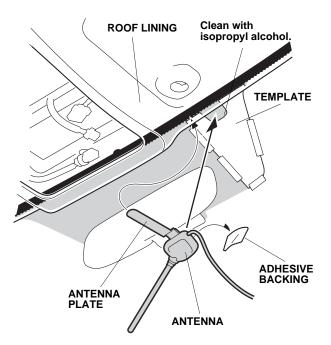
28. Remove the adhesive backing from the antenna. Insert the antenna plate behind the roof lining, align the antenna base to the template, and attach the antenna to the windshield. Apply pressure to the antenna base to make sure it sticks to the windshield.
