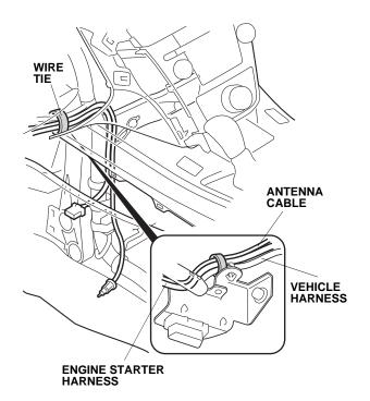
63. At the right kick panel (removed in step 21), slide the holder on the engine starter subharness 34-pin connector onto the holder lock on the vehicle 6-pin connector.
