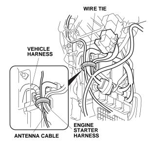
59. Route the engine starter harness 12-pin connector and antenna cable along the dashboard frame towards the center console.
