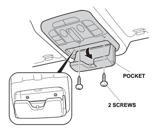
6. Using a plastic trim tool, remove the roof console (two clips and unplug three vehicle connectors).
