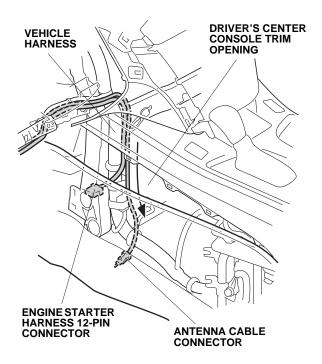
61. Secure the engine starter harness and antenna cable to the dashboard frame with three wire ties.
