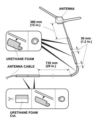
23. Using scissors, cut one urethane foam piece in half. Wrap the two halves of the urethane foam around the antenna cable at the measurements shown.
