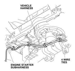
71. Behind the center console, secure the engine starter subharness to the vehicle harness with one wire tie.
