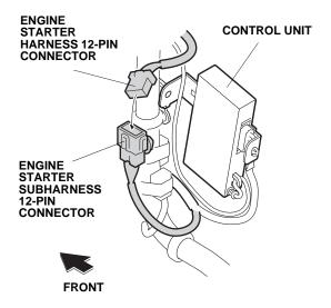
76. Install the engine starter control unit bracket to the vehicle bracket using a flange bolt.
