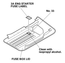
82. Using isopropyl alcohol on a shop towel, clean the area where the caution label will attach. Attach the caution label to the under side of the hood as shown.
