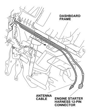
60. Route the engine starter harness 12-pin connector and antenna cable connector down along the vehicle harness to the driver's center console trim opening.
