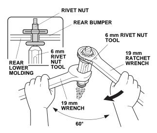
13. Remove the rivet nut tool from the rivet nut by turning the tool body in a counterclockwise direction.
