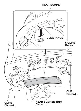
3. Install the rear lower molding to the rear bumper with six clips.
