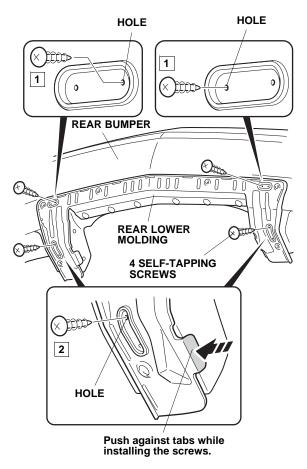
6. Push on the outside edge of the rear lower molding to make sure there is no gap.
