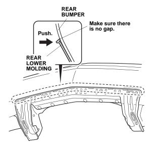
NOTE: If there is a gap at the outside edge of the rear lower molding, remove the self-tapping screws and realign the rear lower molding. Repeat step 4 to drill in the four alternate locations, and then reinstall the self-tapping screws in the alternate locations.
