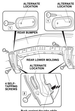
Push against the tabs while installing the self-tapping screws.
