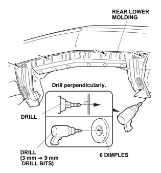
8. Install six rivet nuts in the holes in the positions shown. Follow steps 9 through 13.
