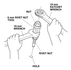
12. Turn the 19 mm ratchet wrench clockwise while holding the tool perpendicular to the work. Turn the nut until firm resistance is felt. Several turns will be required.
