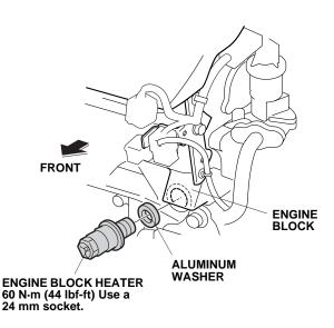
21. Plug the connector end of the heater harness into the engine block heater.
