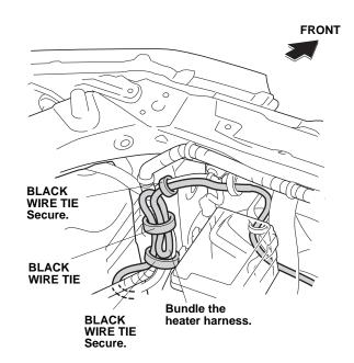
29. Tighten the two black wire ties (loosely installed in step 24).
