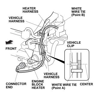
22. Route the heater harness as shown and secure the heater harness to the vehicle harness using one white wire tie (point A). Secure the heater harness to the vehicle harness with another white wire tie (point B).
