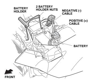
9. Remove the battery and the battery box.
