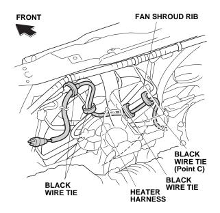
24. Continue routing the heater harness through the engine compartment. Loosely secure it to the vehicle harness with two black wire ties.
