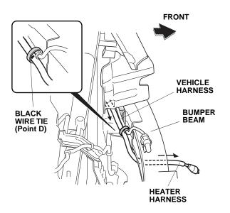
27. Secure the heater harness to the vehicle harness with one black wire tie.
