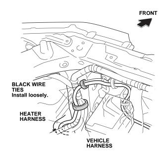
25. Route the heater harness through the opening in the front bulkhead.
