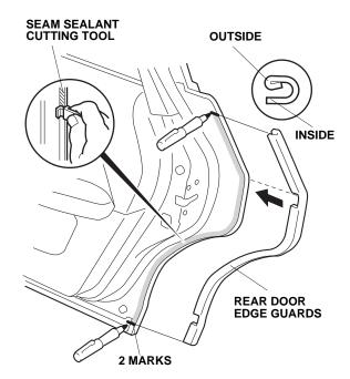
4. Position the cutting edge of the seam sealant cutting tool against the door edge and trim the seam sealant from mark to mark.
