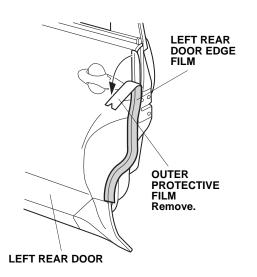
20. Starting in the middle of the door edge film and working outward, use your fingers to fold the door edge film around the edge of the left rear door. Move your fingers in one direction. Attach the door edge film over the seam sealant. Do not trim or damage the seam sealant.
