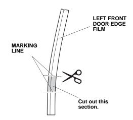
6. Partially peel back the adhesive backing from the upper part of the left front door edge film. Align the V-notch in the upper part of the door edge film with the end of the character line on the driver's door.
