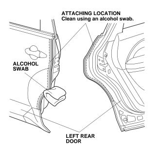
15. Close the left rear door. Using a spray bottle with 3M protective tape application solution, spray the area where the door edge film will attach.
