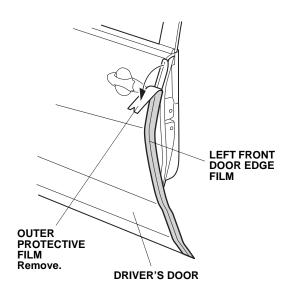
11. Starting in the middle of the door edge film and working outward, use your fingers to fold the door edge film around the edge of the driver's door. Move your fingers in one direction. Attach the door edge film over the seam sealant. Do not trim or damage the seam sealant.
