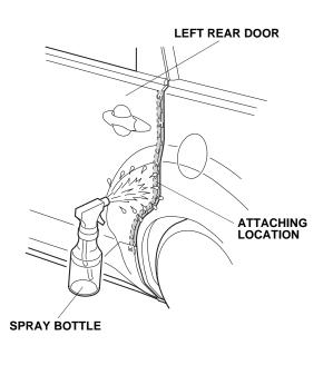
16. Open the left rear door again. Peel back about 50 mm (2 in.) of adhesive backing from the left rear door edge film. Align the V-notch in the door edge film with the end of the character line on the upper part of the left rear door.
