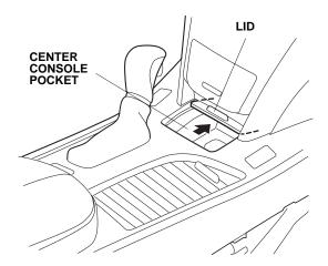
Open the accessory socket lid. Remove the accessory socket by reaching in the driver's console trim opening and pushing up on the accessory socket. Use a 90° awl to release the two retaining tabs.
