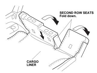
5. Position the cargo liner on the back of the second row seats, and reinstall the headrests.
