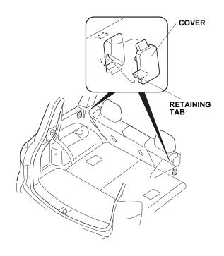
4. Install the cargo cover into the recess in the left rear side panel with the flat side facing up, then compress the cargo cover, and install it in the right rear side panel.
