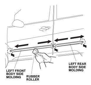
14. Repeat steps 1 thru 13 to install the body side moldings on the right side of the vehicle.
