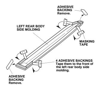
Position the left rear body side molding on the left rear door, and align it with the two marks made in step 8.
