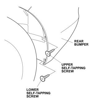
Insert the top edge of the left bracket behind the inner fender, then reinstall the upper self-tapping screw.
