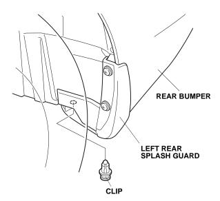
10. Repeat steps 5 through 9 to install the right rear splash guard on the right side of the vehicle.
