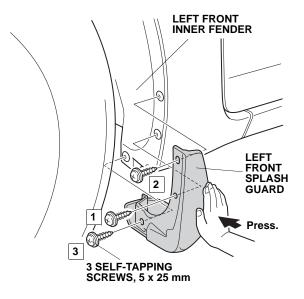
4. Turn the steering wheel fully clockwise, and repeat steps 2 and 3 to install the right front splash guard.
