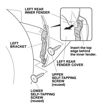
7. Reinstall the lower self-tapping screw.
