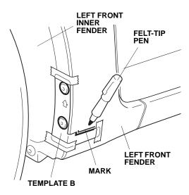
11. Carefully remove template B. Do not damage the template, it is needed to mark the right side of the vehicle.
