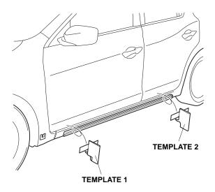
22. Using the palm of your hand, firmly press the rail against the side sill for 30 seconds. Then use a rubber roller to set the adhesive.
