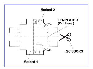
14. Fold each template as shown (Template 1 is used to mark the front of the side sill, and template 2 is used to mark the rear of the side sill.).
