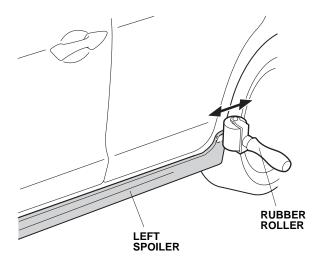
42. Repeat steps 1 through 41 to install the spoiler on the right side of the vehicle.
