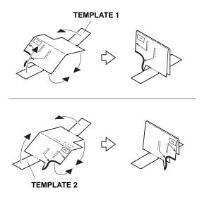
15. Insert the tab on template 1 into the gap between the left front door and the side sill at the measurement shown. With the template flush against the side sill, tape the template to the door. There should be no gap between the template and the side sill.
