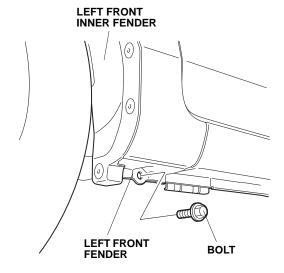
Using a utility knife, remove the undercoating in the area shown.
