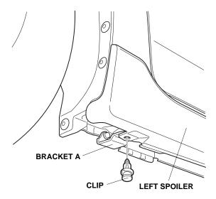
30. Install the clamp to the left spoiler using a bracket screw.
