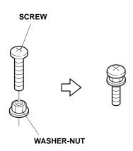
37. Install the screw into the clamp and tighten it securely. Then finger-tighten the washer-nut against the clamp. While holding the screw, tighten the washer-nut.
