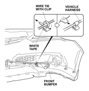
22. Secure the vehicle harness to the front bumper.
