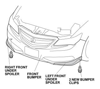
24. Using a rubber roller, apply firm pressure, especially at the ends, to set the adhesive.
