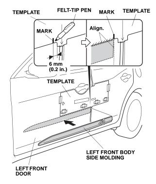
6. Align the left front body side molding with the template and the mark on the template, then attach it to the left front door as shown. Go to step 8.
