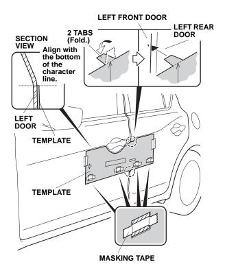
Align the template with the bottom of the character line, and attach the template to the left doors with masking tape as shown. 3. Use two alcohol swabs to thoroughly clean the areas where the left body side moldings will attach.
