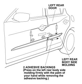
13. Using a rubber roller, apply firm pressure, especially at the ends, to set the adhesive.
