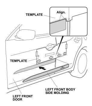
8. Press on the left front body side molding firmly with the palm of your hand while removing about 50 to 100 mm (2.0 to 3.9 in.) of the adhesive backing at a time.
