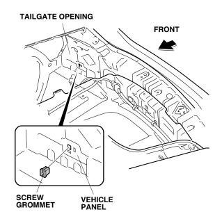
34. Secure the control unit to the vehicle panel with one self-tapping screw.
