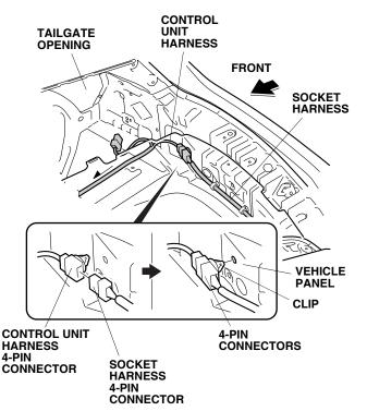
31. Secure the 4-pin connector to the vehicle panel with the clip on the control unit harness 4-pin connector.
