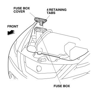
43. Install 7.5A fuses into the #9 and #11 slots in the fuse box. Reinstall the fuse box cover.
