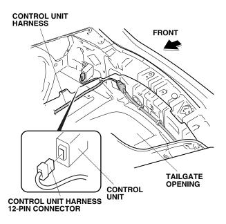
36. Route the control unit harness along the vehicle harness, and secure it to the vehicle harness with four wire ties.
