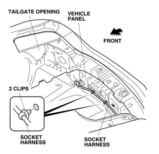
30. Plug the socket harness 4-pin connector into the control unit harness 4-pin connector.
