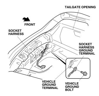
28. Route the socket harness as shown, and secure it to the vehicle panel with the two clips.
