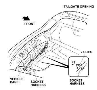
29. Continue routing the socket harness, and secure it to the vehicle panel with the two clips.
