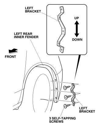
Install the left rear splash guard to the left rear inner fender and left bracket with two 5 x 20 mm selftapping screws and the bolt removed in step 1.
