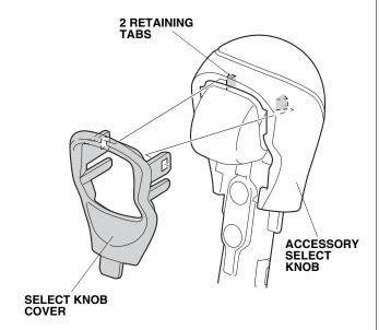
8. Secure the shift boot to the accessory select knob with two retaining tabs.
