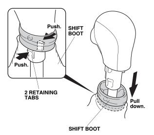
4. Remove the select knob cover (two retaining tabs).
