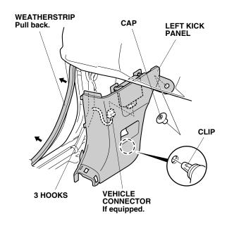
25. Remove the driver's console side trim (nine clips and unplug the vehicle connector, if equipped).
