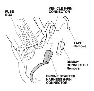
45. Secure the 6-pin connector from step 44 to the vehicle harness with one wire tie.
