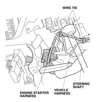
60. Route the engine starter harness as shown. Secure the engine starter harness at the white tape to the vehicle harness at the vehicle clip with one wire tie.
