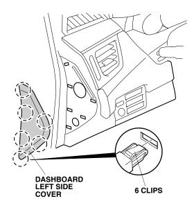
22. Remove the driver's under cover (turn the knob, three clips, two pins, two harness clips, and unplug the vehicle connectors).
