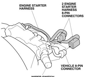
64. Secure the engine starter harness to the vehicle harness with three wire ties.
