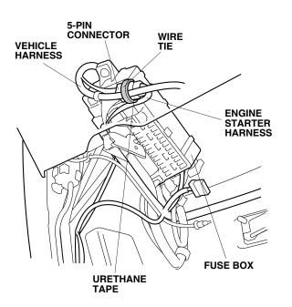
51. Remove the vehicle ground bolt, then use it to secure the engine starter harness ground terminal to the vehicle.
