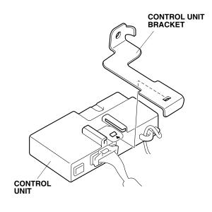
57. Remove the vehicle nut from the vehicle bracket, and secure the control unit bracket to the vehicle bracket with the vehicle nut just removed. Torque the vehicle nut to: 18.7 ~ 24.5 N·m (13.8 ~18.1 lbf·ft). NOTE: Make sure the tab on the control unit bracket
