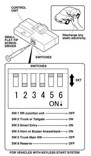
11. Using a small flat-tip screwdriver, set the switches on the control unit as shown. Go to step 14.
