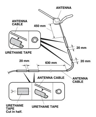
30. Cut one urethane tape in half. Wrap the two cut pieces of urethane tape around the antenna cable at the measurements shown.
