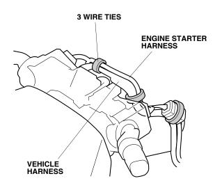
68. Unplug the vehicle 2-pin connector, and plug it into the engine starter harness 2-pin connector. Plug the remaining engine starter harness 2-pin connector into the vehicle 2-pin connector.
