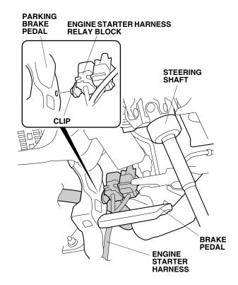
53. Secure the engine starter harness to the vehicle harness with three wire ties.
