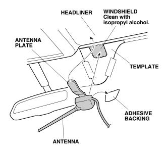
32. Remove the adhesive backing from the antenna. Insert the antenna plate behind the headliner, align the antenna to the template, and attach the antenna to the windshield as shown.
