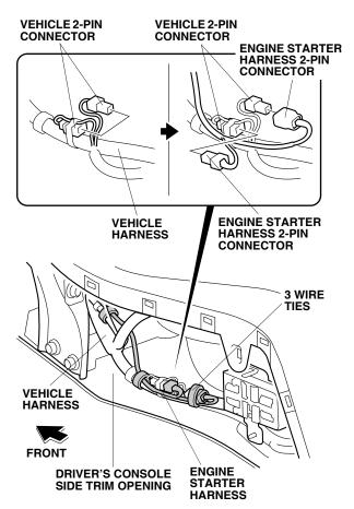
69. Secure the engine starter harness to the vehicle harness with three wire ties as shown.
