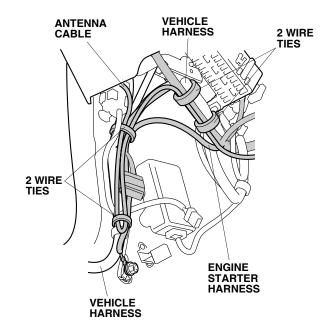
59. Route the engine starter harness and secure it to the vehicle harness with two wire ties.
