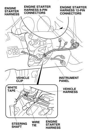
61. Secure the engine starter harness to the vehicle harness with one wire tie.
