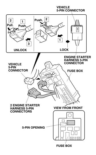
50. Secure the 5-pin connector to the vehicle harness with one wire tie.
