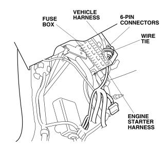
46. Route the engine starter harness along the vehicle harness as shown.
