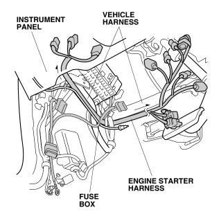
47. Unplug the vehicle 20-pin connector from the fuse box, and plug it into the engine starter harness 20-pin connector. Plug the remaining engine starter harness 20-pin connector into the 20-pin opening in the fuse box.
