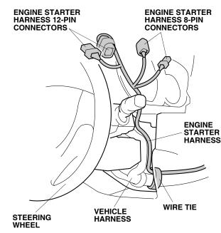
62. Unplug the vehicle 12-pin connector from the light/ turn signal switch, and plug it into the engine starter harness 12-pin connector. Plug the remaining engine starter harness 12-pin connector into the light/turn signal switch.
