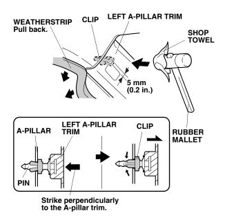
19. Pull back the weatherstrip, and remove the left A-pillar trim (one clip and unplug the vehicle connector).
