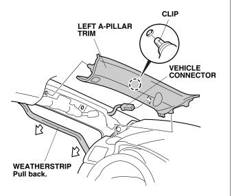
20. Remove and discard the clip from the left A-pillar trim, and install a new pillar clip (supplied).
