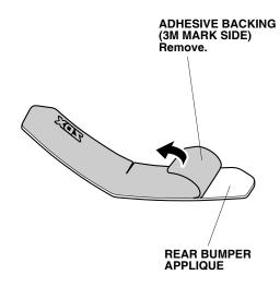
4. Spray the rear bumper applique with the protective tape application solution.
