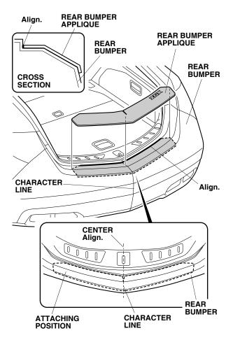
6. Align and attach the rear bumper applique to the rear bumper as shown.
