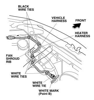
13. Secure the heater harness to the fan shroud rib and vehicle harness with three white wire ties and two black wire ties.
