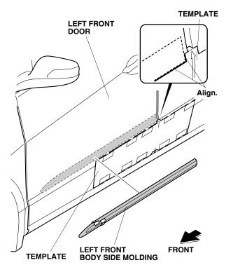
Peel back approximately 1½ to 2 inches of adhesive backing from each adhesive strip, and tape the ends to the front surface of the body side molding. Remove the small end pieces of adhesive backing.
