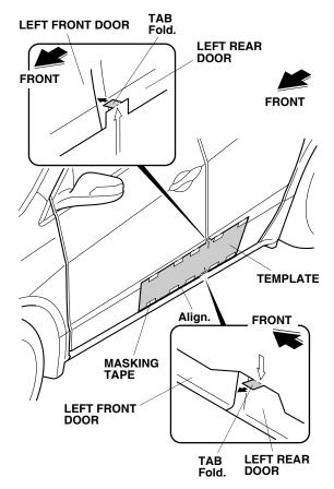
3. Align the template to the left front door and left rear door and attach it with pieces of masking tape as shown.
